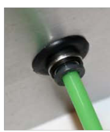
Backside View of Fitting installed in Grommet
