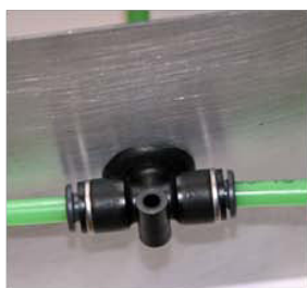
Front Side view of Union Tee Installed in Grommet
